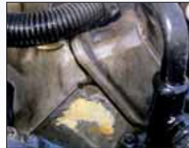
"Fixed" valve cover leak.
