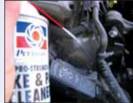
Clean area with Permatex® Brake & Parts Cleaner.
