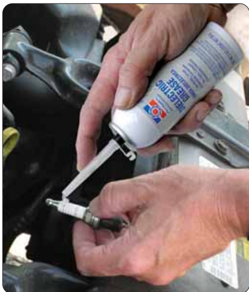
Apply Permatex® Dielectric Grease to ceramic part of spark plug.
