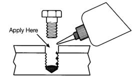
7 Assemble and tighten as usual. When tightening to . established torque values, torque compensation is not required.
