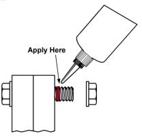
For Blind Holes, apply by dripping several drops of ScrewGlue onto the female threads of the hole. As threads are engaged, compressed air forces the product upwards into the threads.
